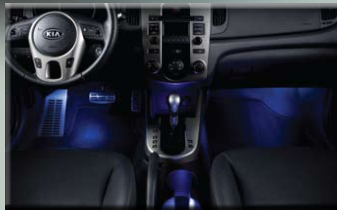
Interior Lighting This fully integrated lighting system allows you to control a set of colored lights within the vehicle. Lights are installed in the cup holders, forward tray and front foot wells. Refer to your dealership for availability. U8680 1M000
